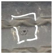
Marks such as these indicate the object has been in the tyre for some time prior to failure =>
