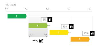
Relationship between tyre RRC grade and vehicle fuel consumption. Results based on VECTO's long haul cycle for default tractor/trailer combination.
